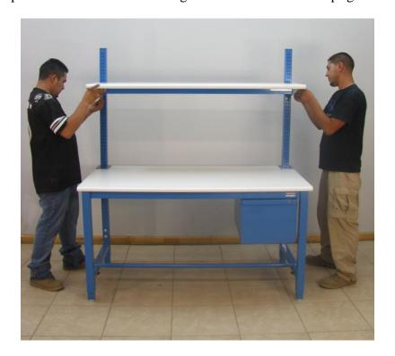
**3.** Tap the shelf top near the uprights to slip the fingers down into position. It doesn't take much of a tap, and can be done with a closed hand.
